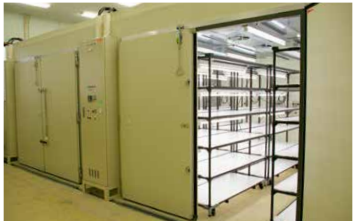
○ Artificial light type raising seedling apparatus (Type 6)
